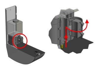
3. Remove the soap container by gently pulling it out of the pump housing.
