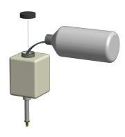
7. Mount the pump housing by gently sliding it back into the slot
