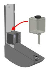
2. Remove the soap container by gently pulling it out of the pump housing.
