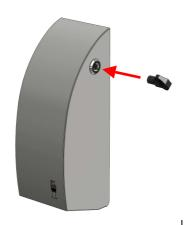
Mount the soap container by gently pushing it into the groove on the pump housing.
