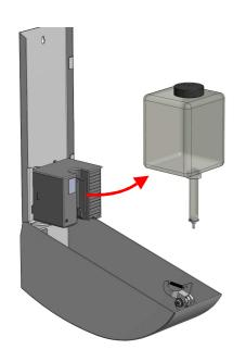
Remove the cap and fill the soap container with appropriate liquid soap.
