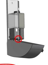
Make sure that the collar is located under the pump housing. —
