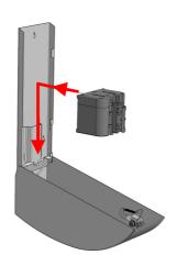
Mount the soap container by gently pushing it into the groove on the pump housing.
