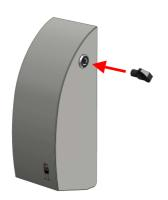
4. Remove the cap and fill the soap container with appropiate liquid soap. Refit the cap and wipe any spilled soap.
