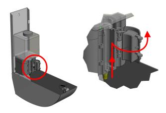
5. Mount the soap container by gently pushing it into the groove on the pump housing.
