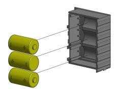
4. Slide the battery box back into the pump housing and gently push it until your hear a "click"
