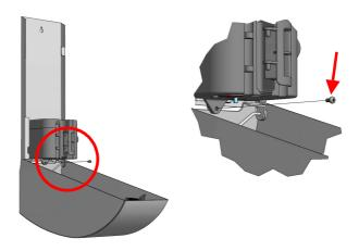
Remove the pump housing by gently lifting it a few centimeters up and then pull it out of the slot.
