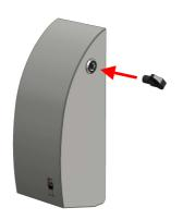
2. Open the flap on the front of the pump housing by gently lifting it approximately 1 cm and turn it anti clockwise.
