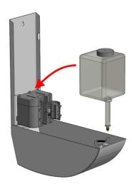
3. Remove the soap container by gently pulling it out of the pump housing.
