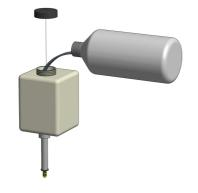
Pull silicone tube downwards and place the outlet nozzle in the slot. Make sure that the collar is located under the pump housing.
