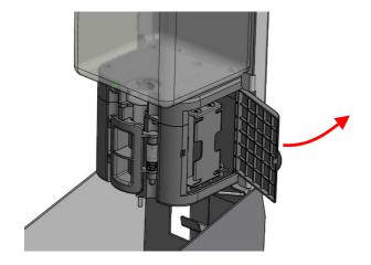
Carefully remove the battery box from the pump housing. Be careful not to pull the wires. Replace the four AA batteries. Be aware that they must be properly oriented with polarity as indicated inside the battery box.
