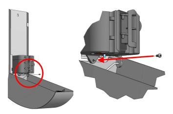
11. Pull silicone tube downwards and place the outlet nozzle in the slot. Make sure that the collar is located under the pump housing.
