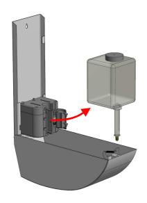
6. Pull silicone tube downwards and place the outlet nozzle in the slot. Make sure that the collar is located under the pump housing.
